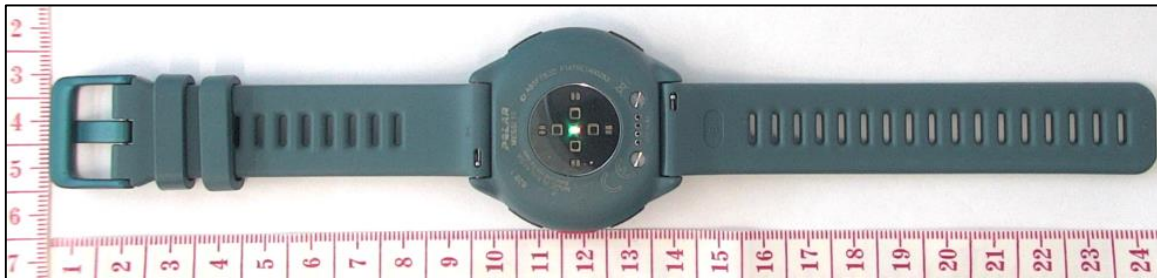
Figure 2. Device from behind, OHR and USB charging cable contacts visible.
