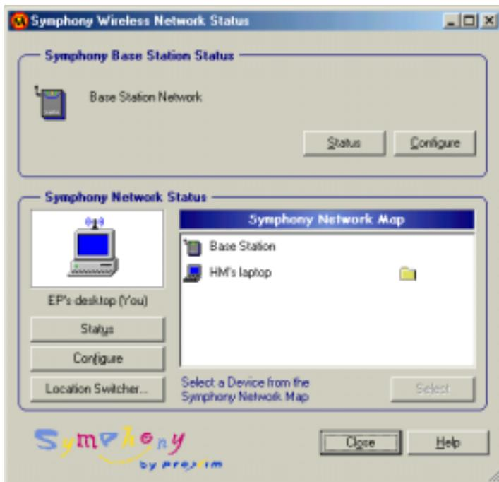
The Maestro has two functions: it monitors the current state of the wireless network and it allows the user to reconfigure network parameters.
