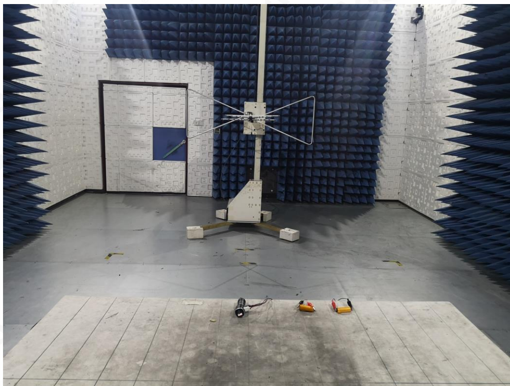
RADIATED EMISSION TEST SETUP ABOVE 1GHZ
