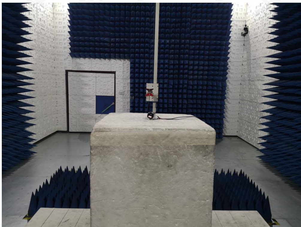
RADIATED EMISSION TEST SETUP ABOVE 1GHZ
