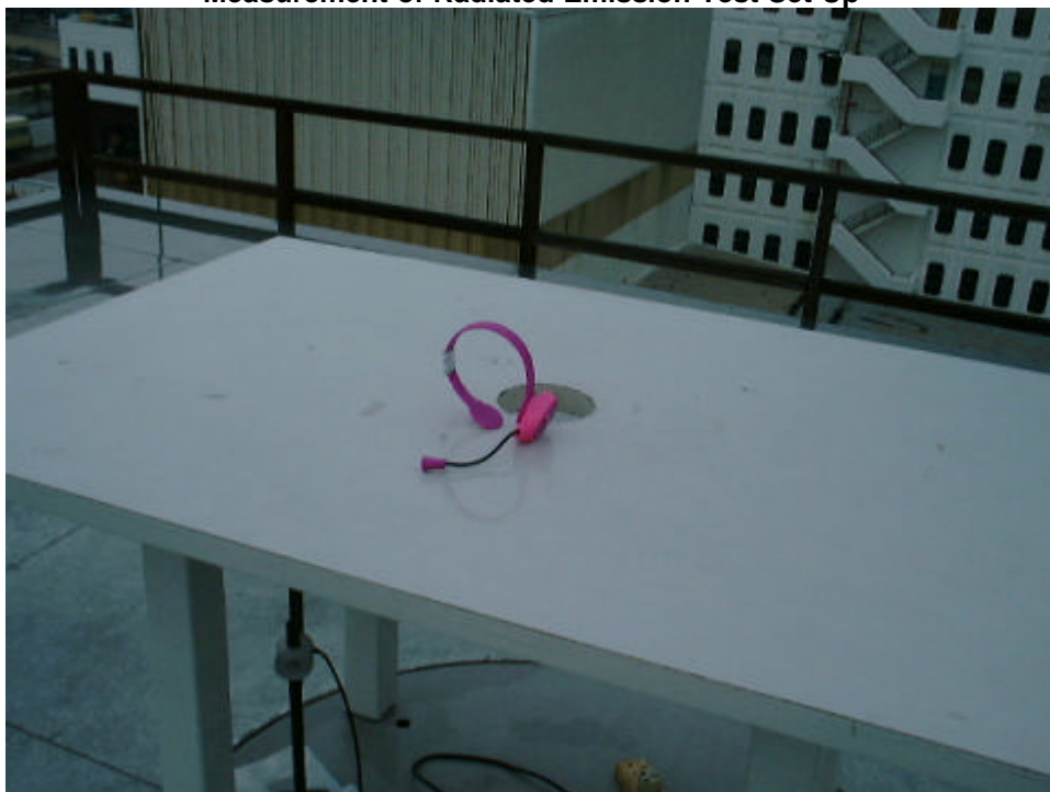
Measurement of Radiated Emission Test Set Up
