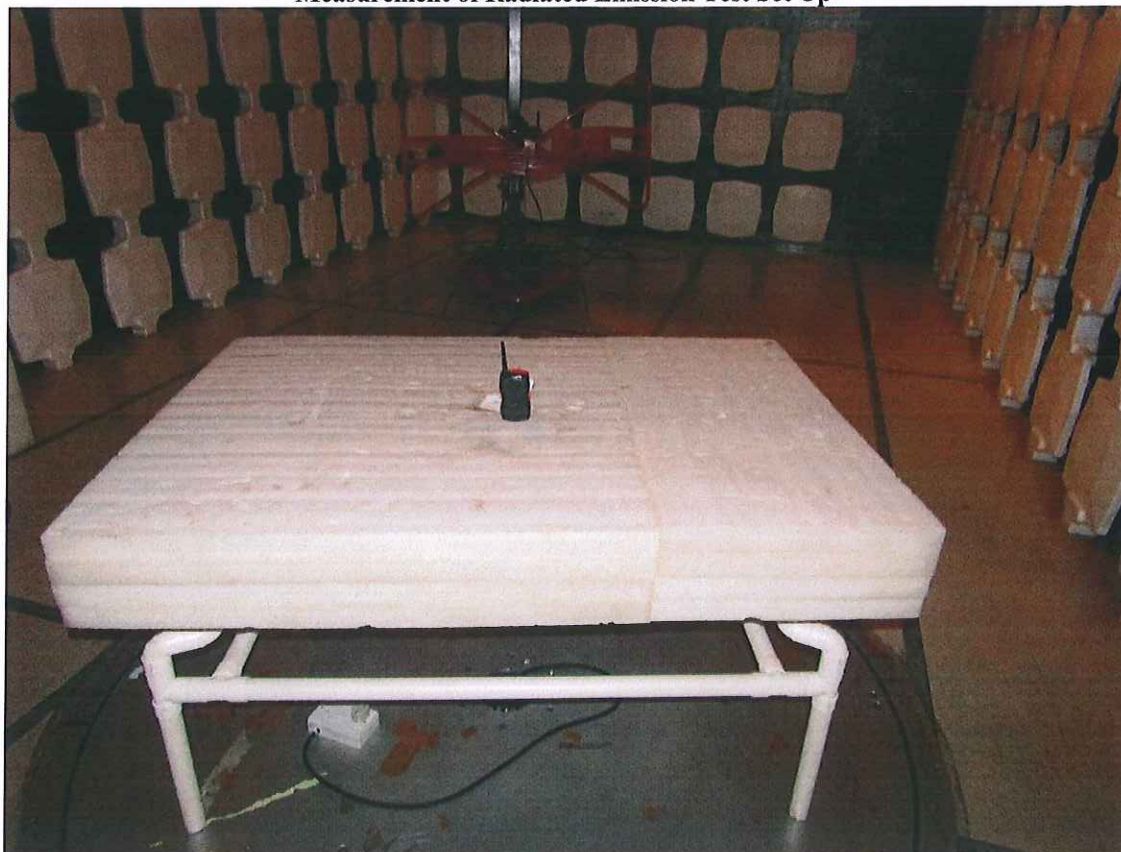
Measurement of Radiated Emission Test Set Up
