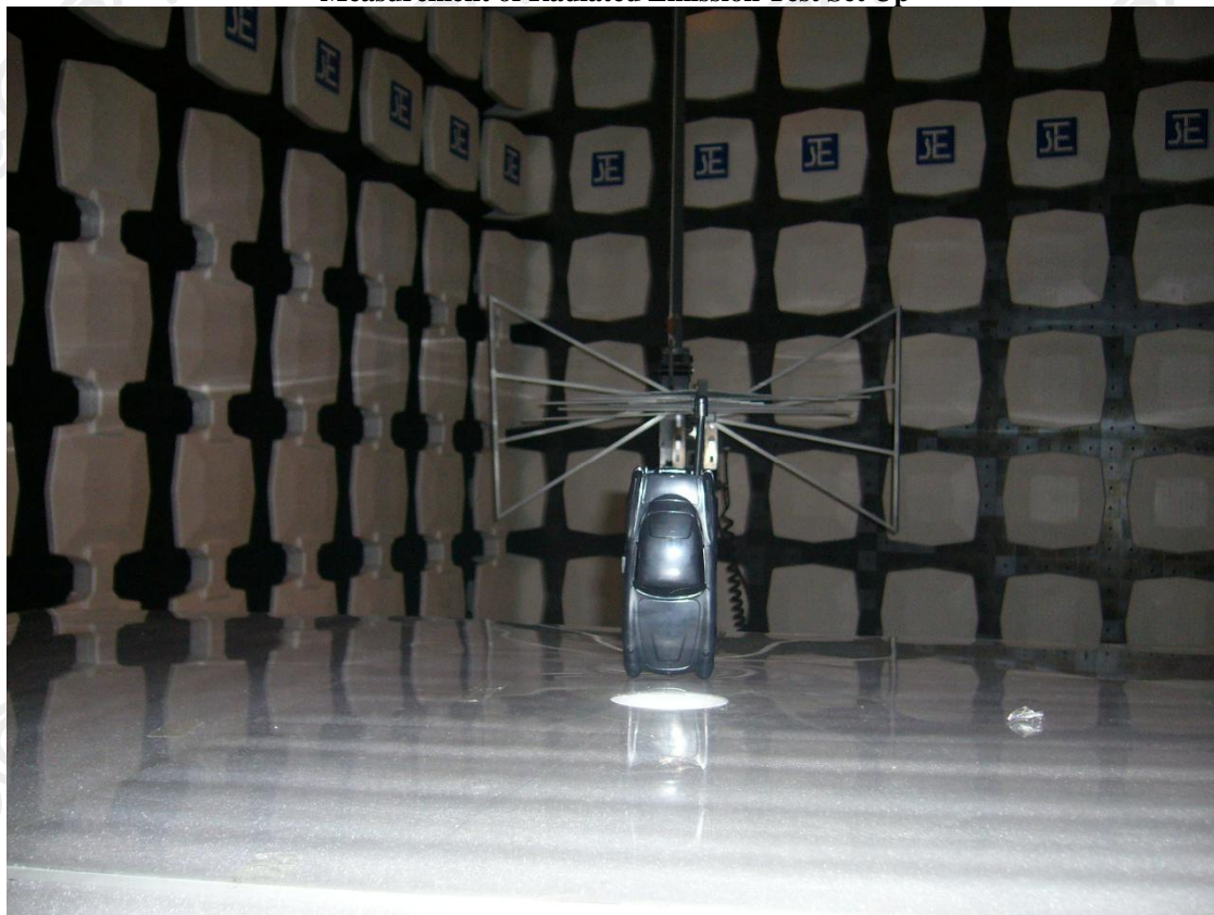
Measurement of Radiated Emission Test Set Up
