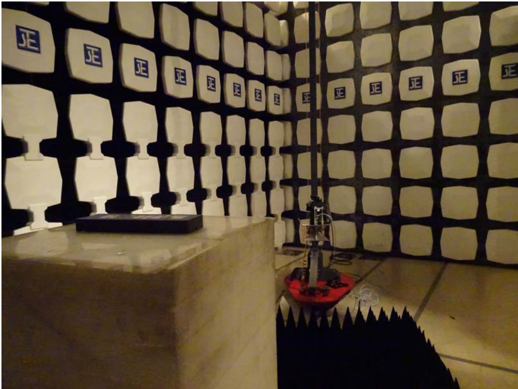
Measurement of Radiated Emission Test Set Up
