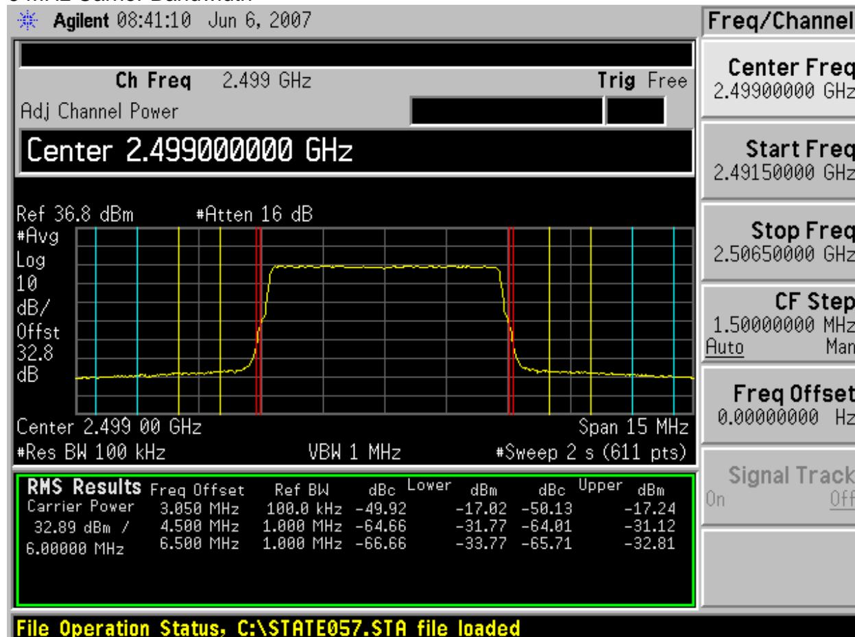
**Test Data – Spurious Emissions at Antenna Terminals**
