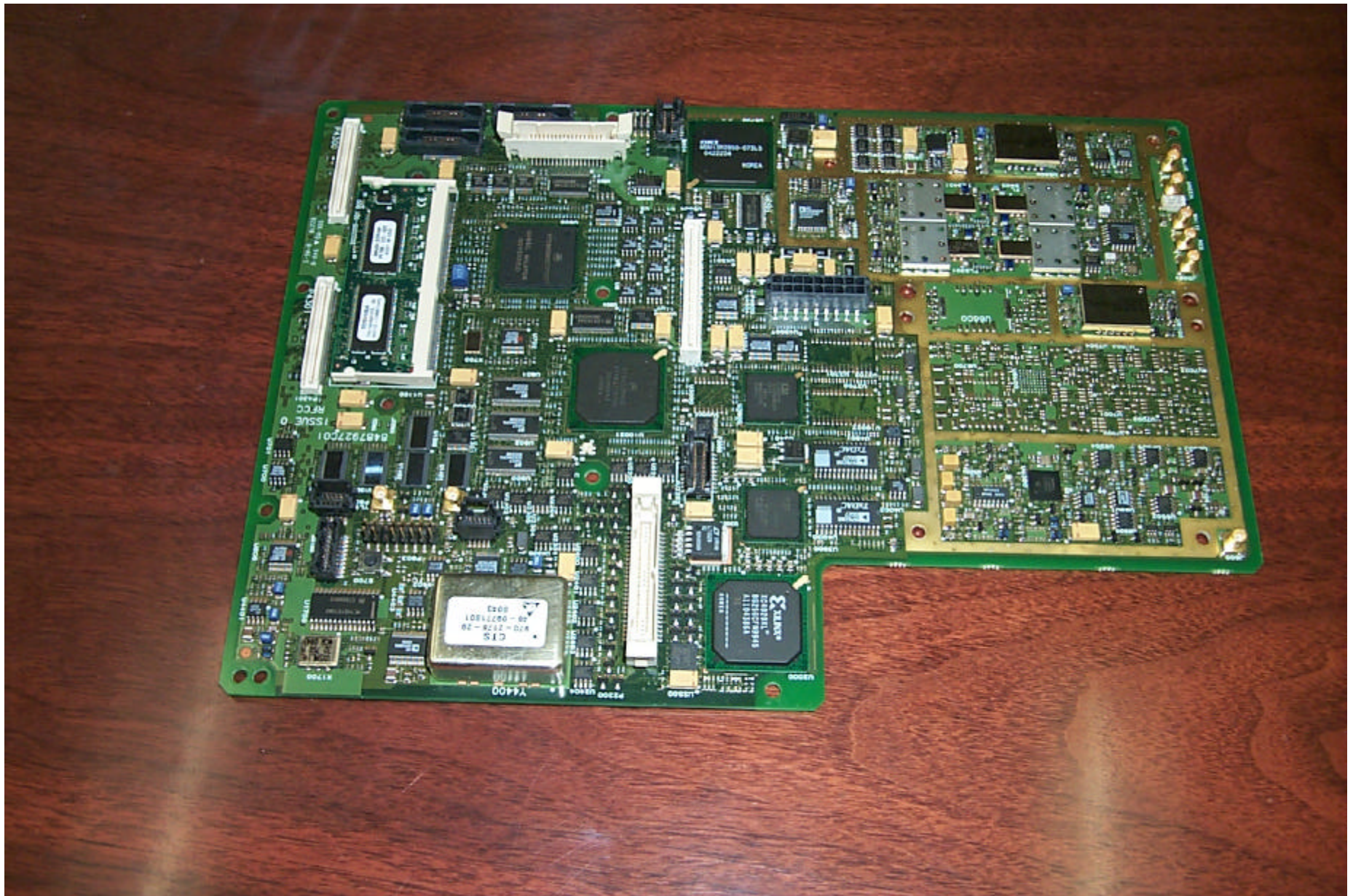
IHET5AP1 SC300 Microcell @ 800MHz RFCC Board - Front View
