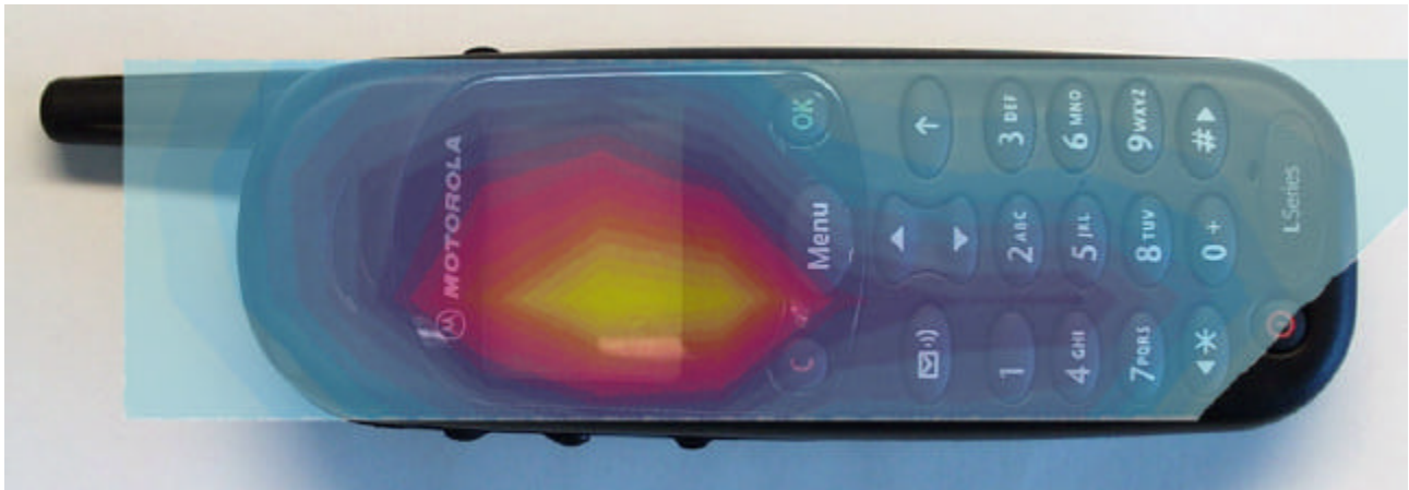
Figure 4. Contour Plot Overlaid on Face of Phone.
