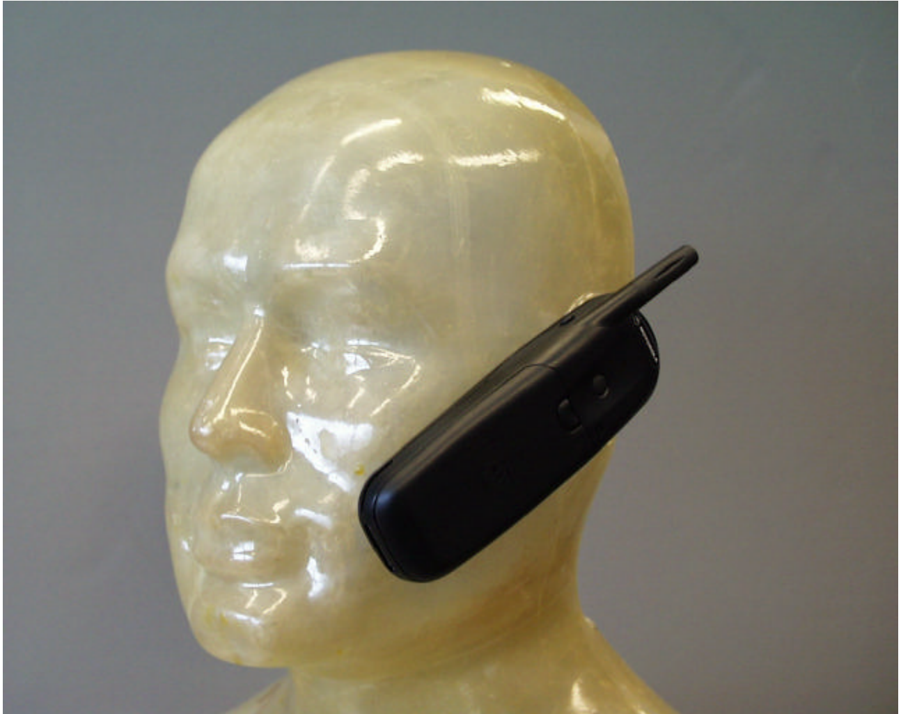
Figure 2. Phone against side of Phantom Head.
