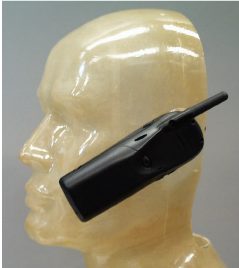
Figure 3. Phone against side of Phantom Head.
