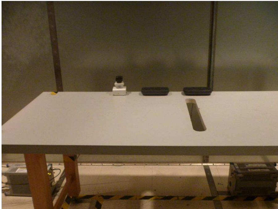
Test Setup Photo – Conducted Emission
