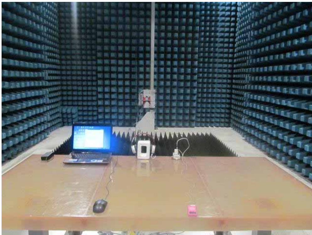
Description: Radiated Emission Test Setup for 1~18GHz
