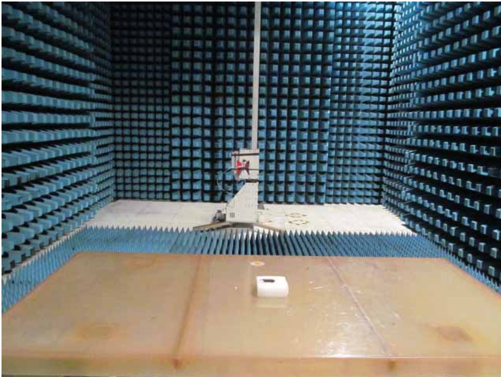
Description: Radiated Emission Test Setup for 1~18GHz
