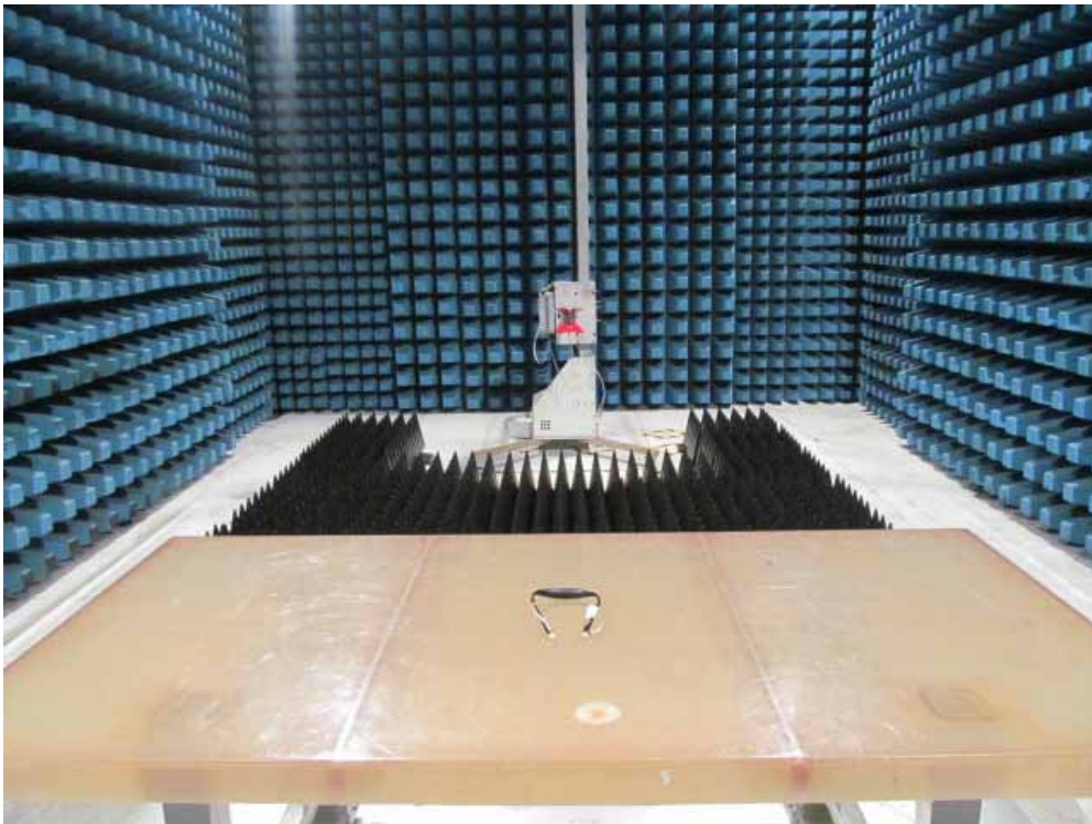
Description: Radiated Emission Test Setup for 1~18GHz
