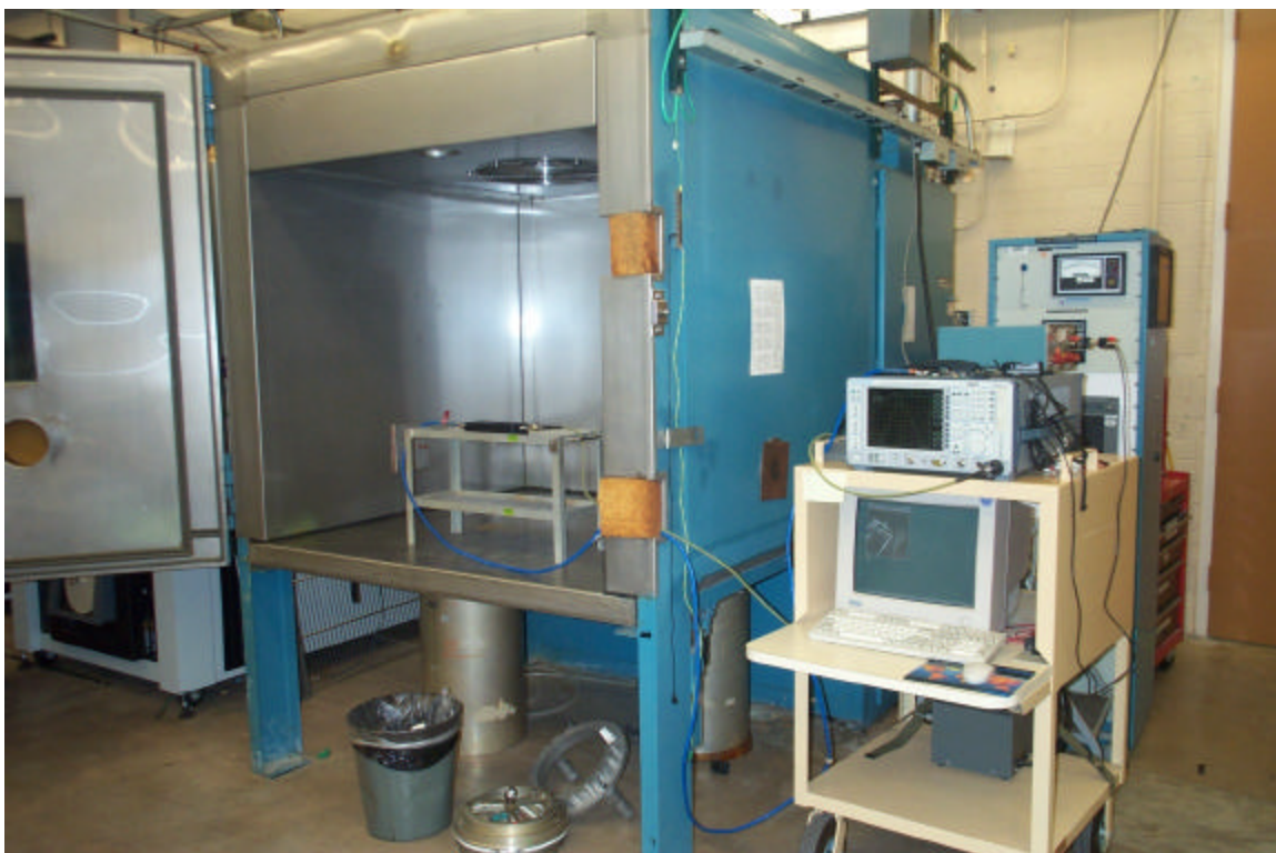
Figure 7.0-7 Frequency Stability versus Temperature Test Setup
