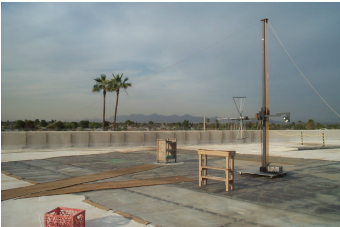
Figure 7.0-6 Radiated Emissions Test Setup -OATS
