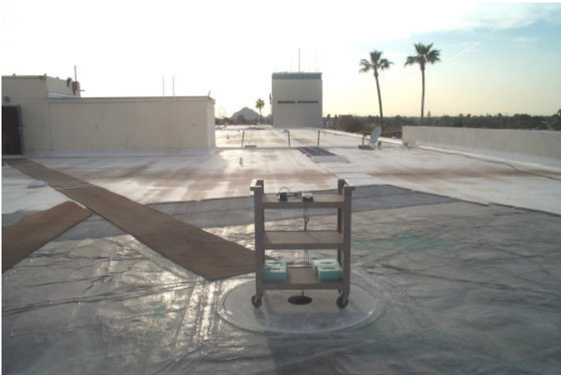
Figure 7.0-5 Radiated Emissions Test Setup -OATS
