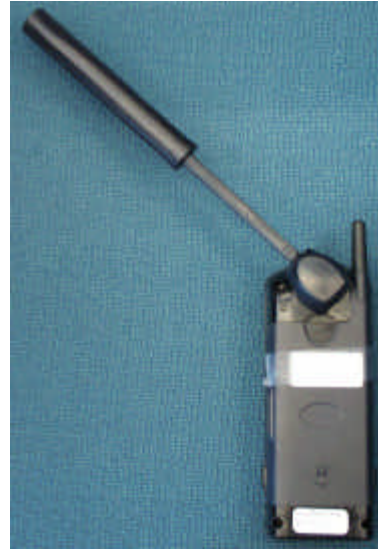
Figure 2. Back of Transceiver Showing Antenna Extended and Cellular Phone Module Installed
