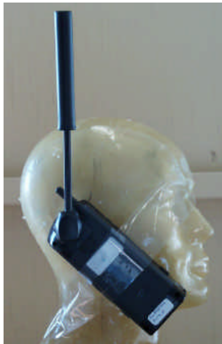
Figure 3. Portable Satellite Transceiver With Portable Cellular Module Installed Against Phantom Head.
