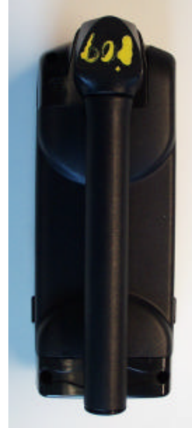
Figure 2. Back of Transceiver Showing Stowed Antenna
