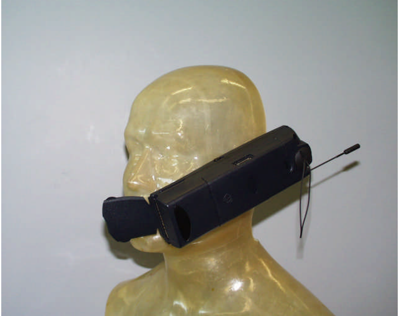
Figure 7. Test position with antenna extended
