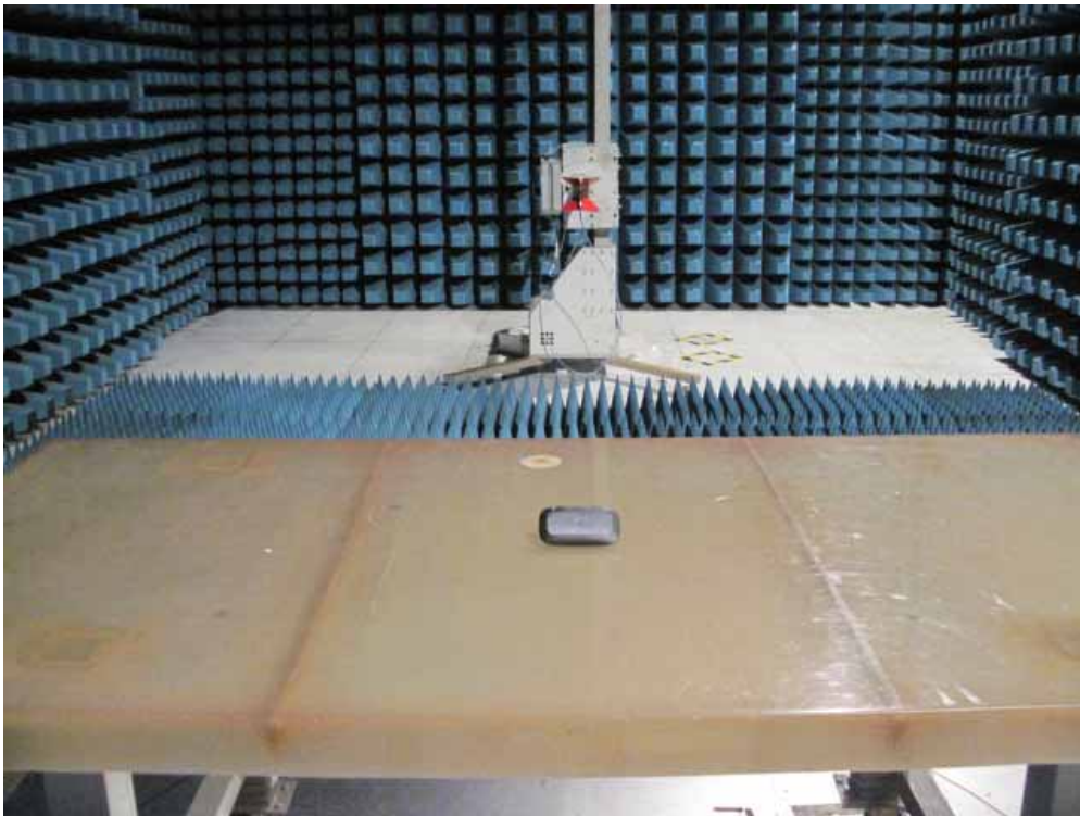
Description: Radiated Emission Test Setup for 1~18GHz
