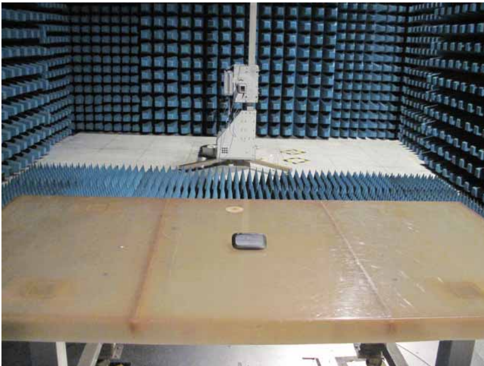
Description: Radiated Emission Test Setup for Above 18GHz
