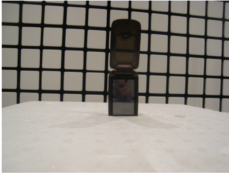
22642-1, IHDT6KH1 placed in test position Z – lid open
