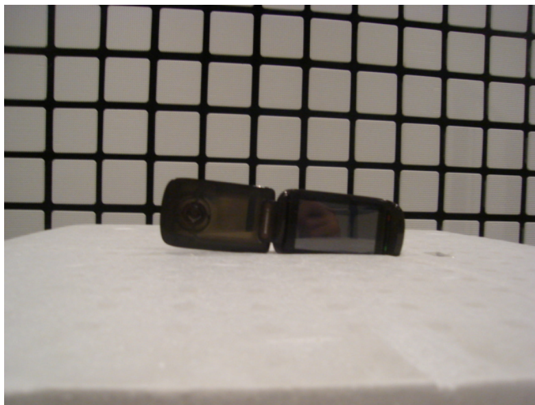
22642-1, IHDT6KH1 placed in test position Y – lid open
