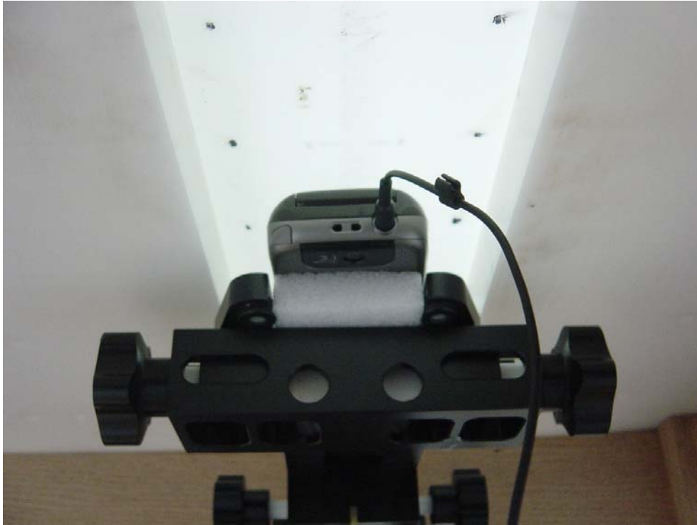
Figure7: Phone Against the Flat Phantom
