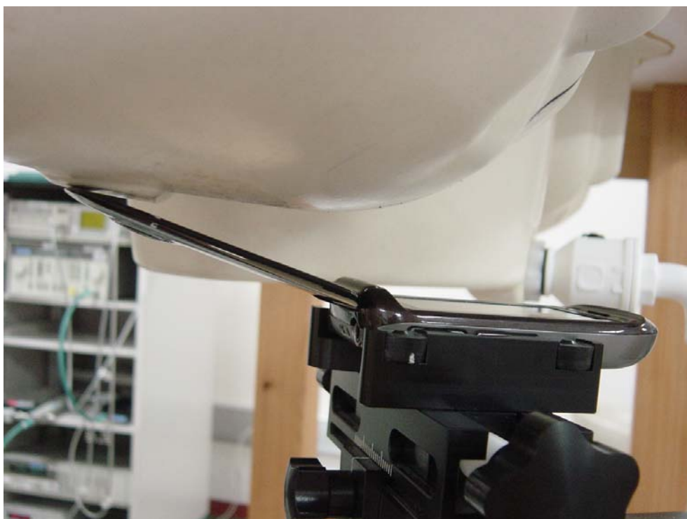
Figure6: Phone Against the Head Phantom (15° Tilt)
