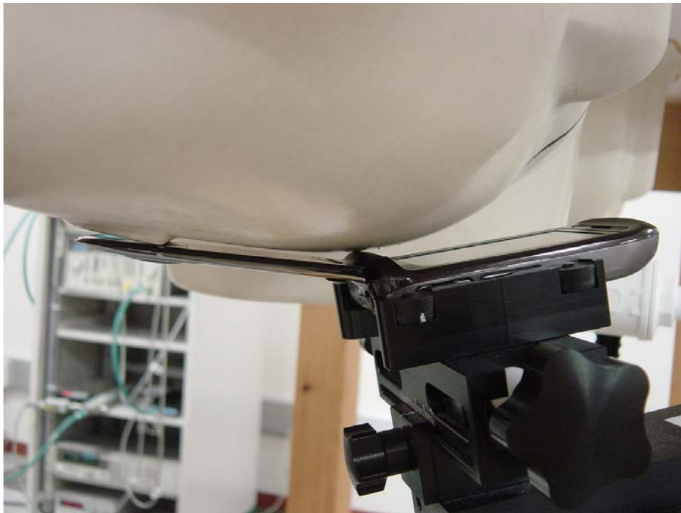
Figure5: Phone Against the Head Phantom (Cheek Touch)
