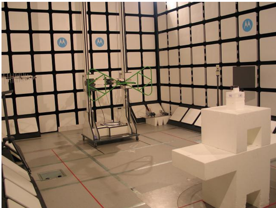
21532-1, IHDT6JG1 setup in semi-anechoic chamber – front view
