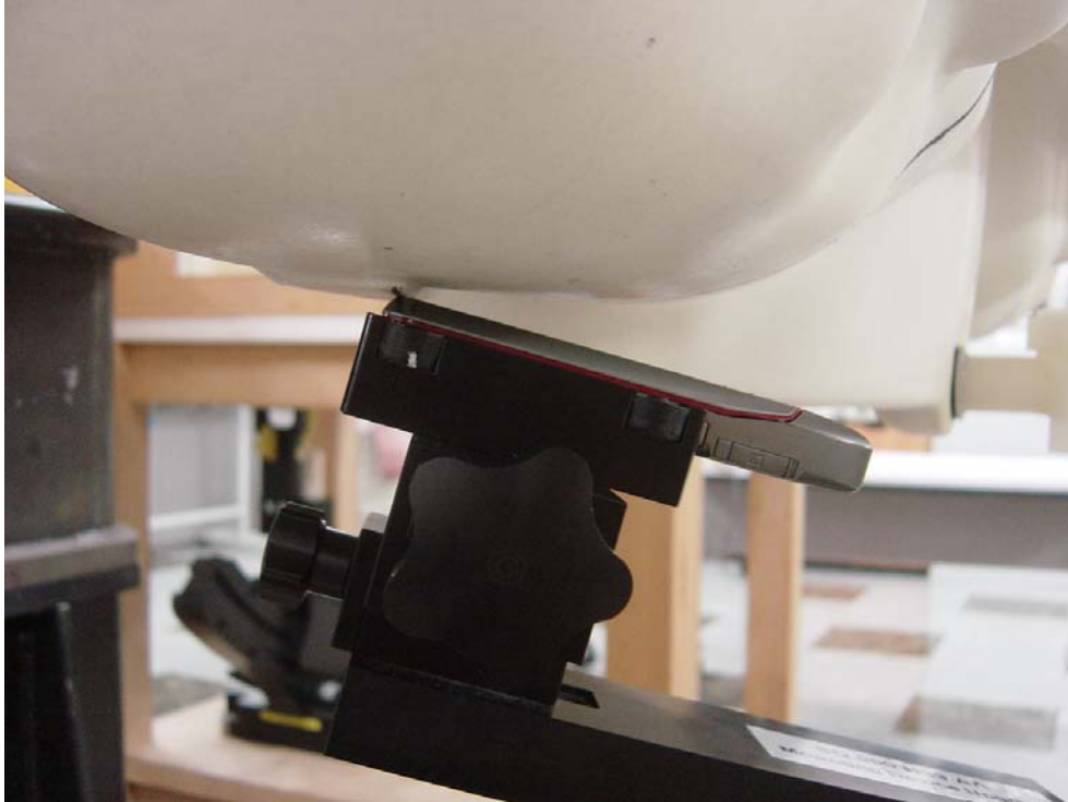
Figure7: Phone Against the Head Phantom (15° Tilt – Slider Closed)
