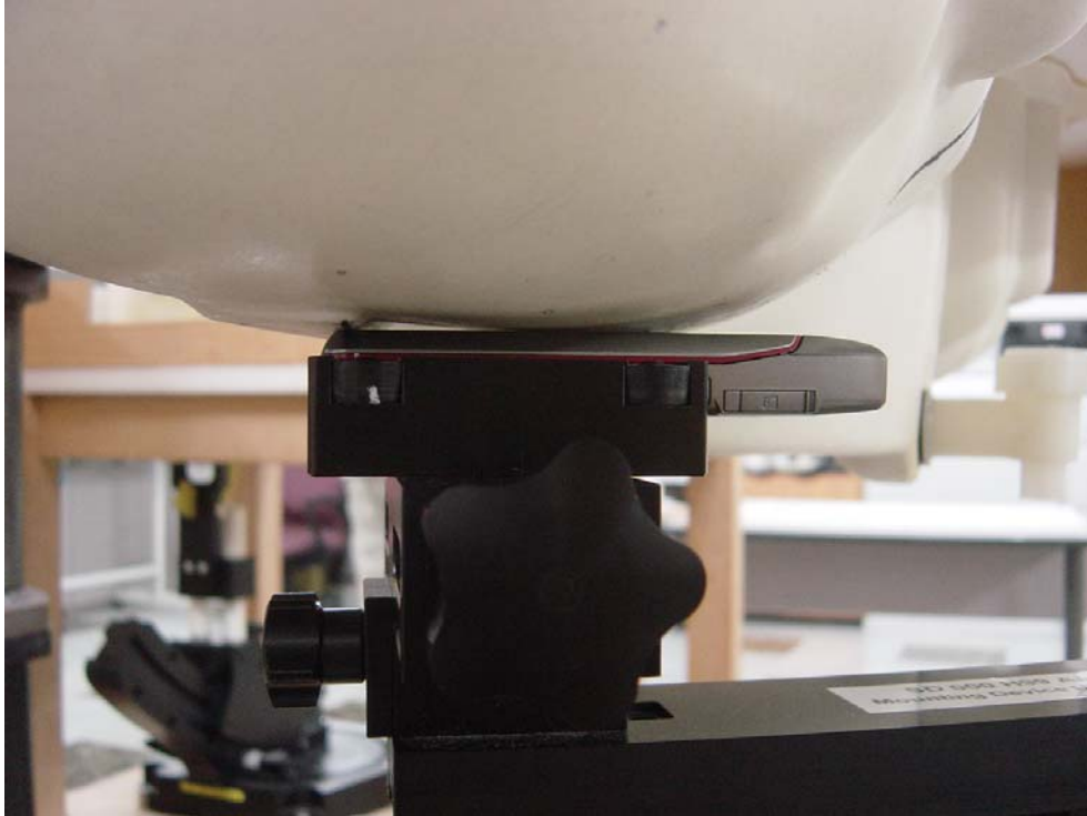
Figure5: Phone Against the Head Phantom (Cheek Touch – Slider Closed)
