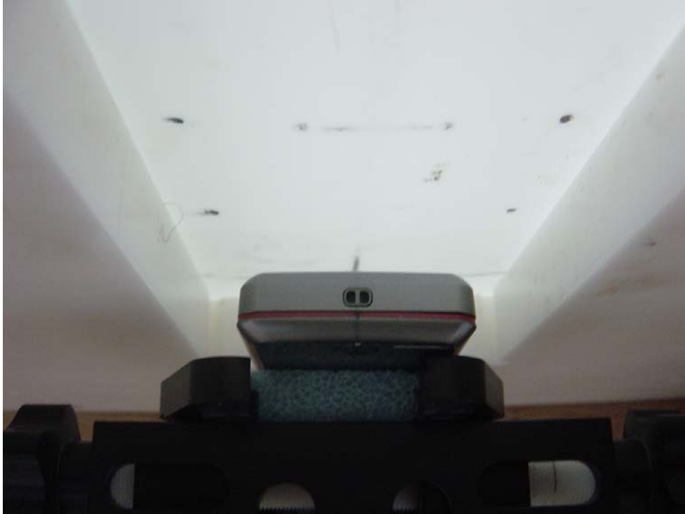
Figure9: Phone Against the Flat Phantom
