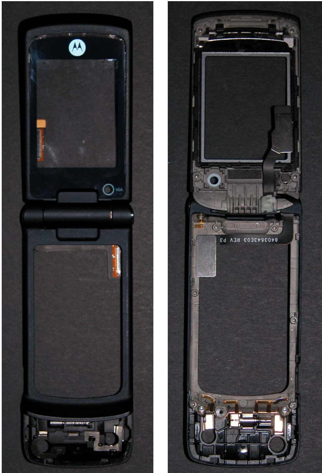
FRONT HOUSING and FLIP INNER HOUSING – External and internal views
