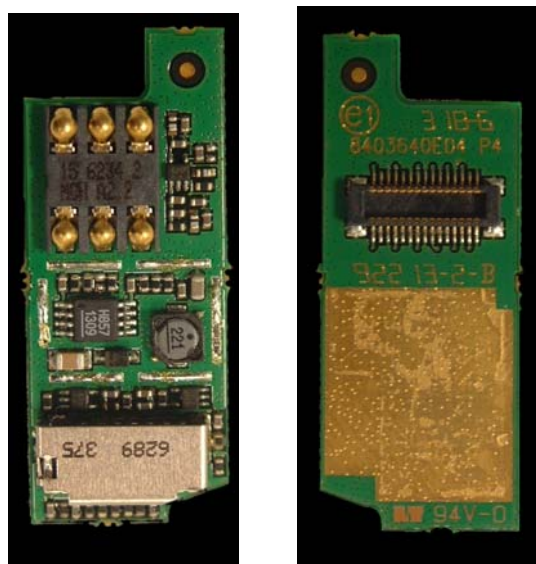
DAUGHTER PCB – Front and Rear views – without shields
