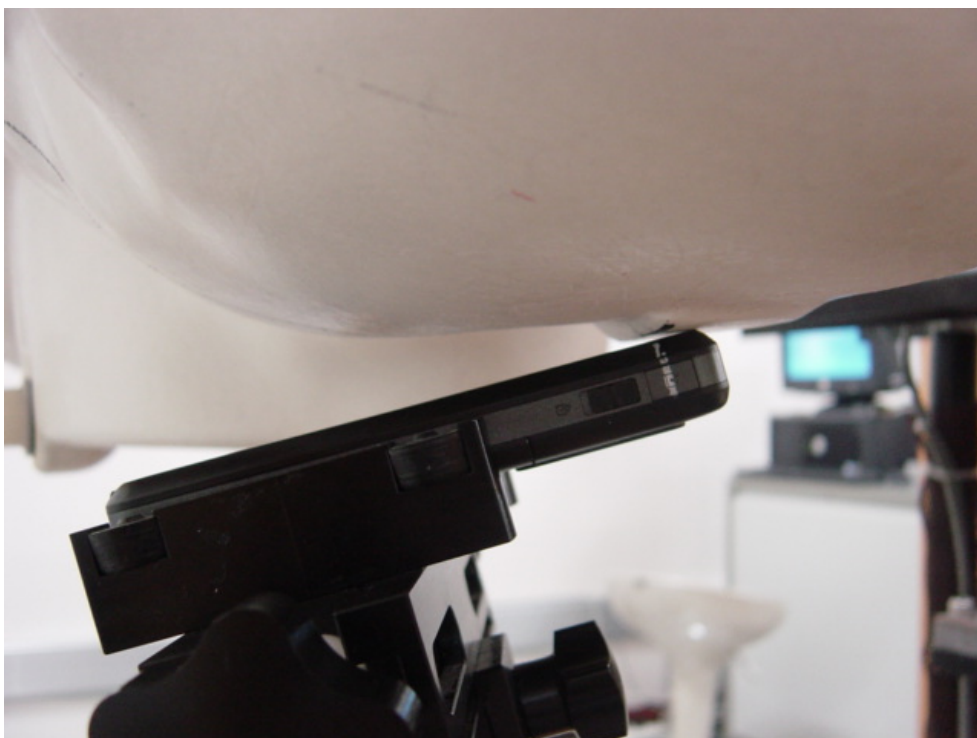
Figure4: Phone Against the Head Phantom (15° Tilt)
