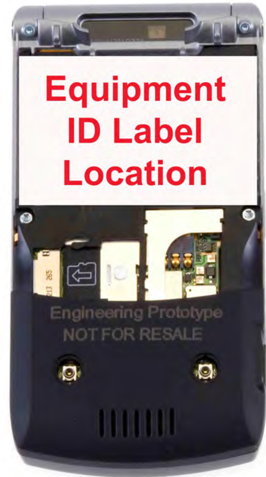
Rear View with Battery Cover Removed Showing ID Label
