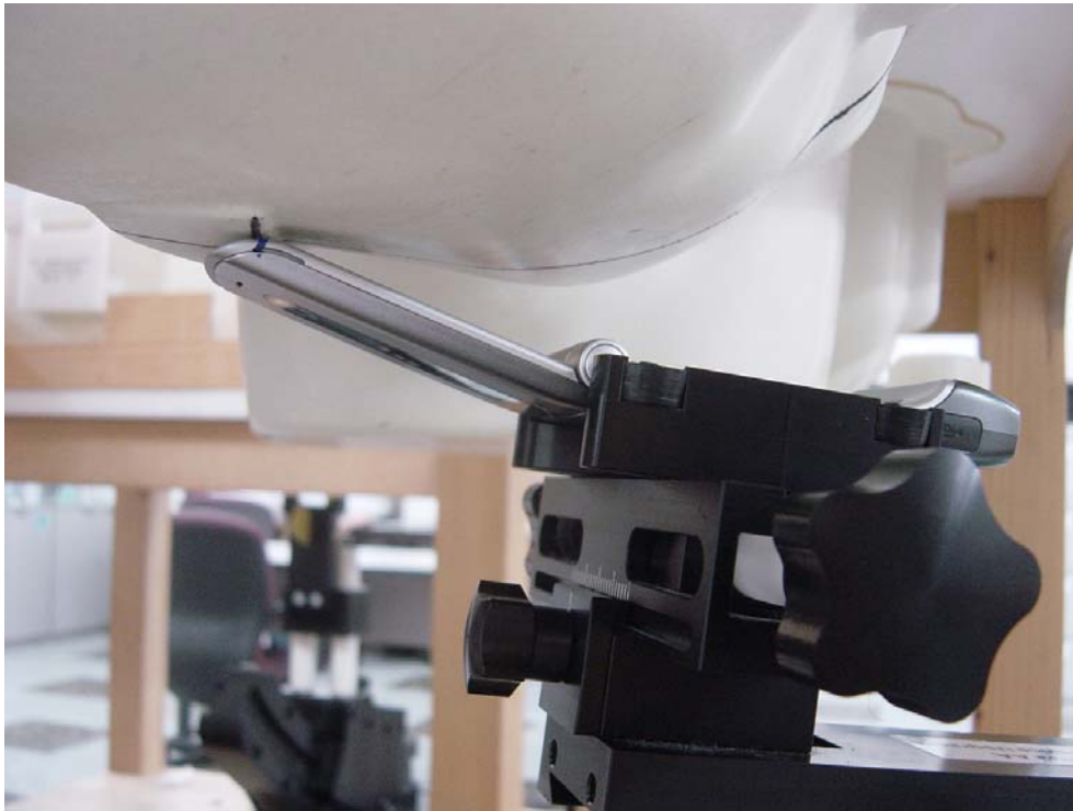
Figure5: Phone Against the Head Phantom (15° Tilt)
