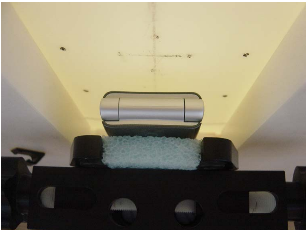
Figure6: Phone Against the Flat Phantom
