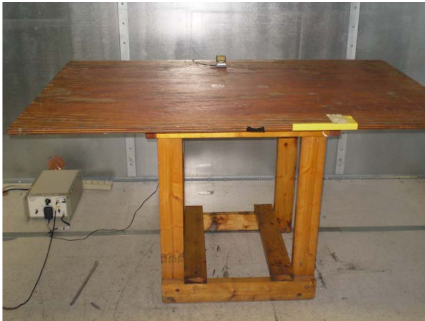
Figure 2. Part 15 AC Line Test Set-Up
