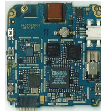
Main PCB (Side B) with shields removed
