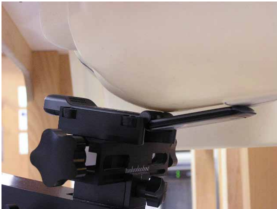
Figure 4. Phone Against the Head Phantom (Cheek Touch)
