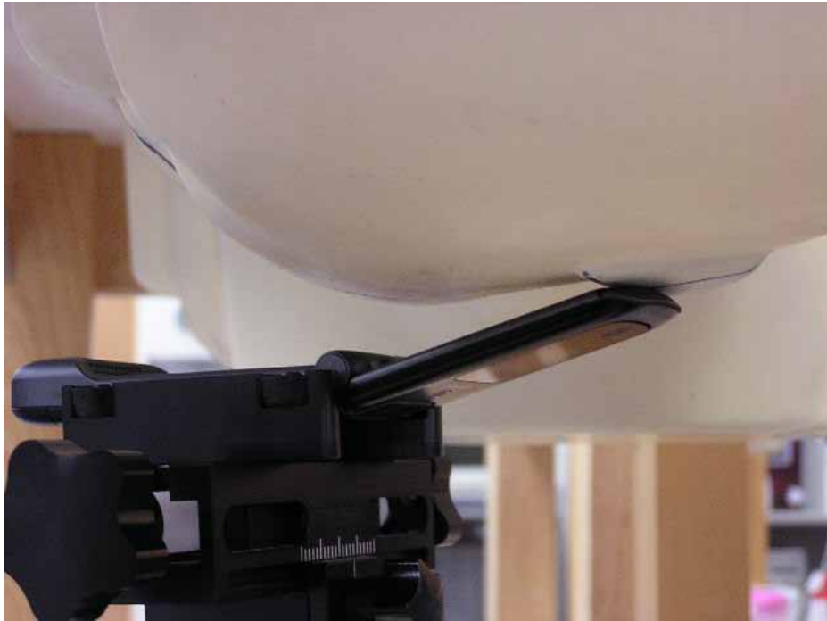
Figure 5. Phone Against the Head Phantom (15°Tilt)
