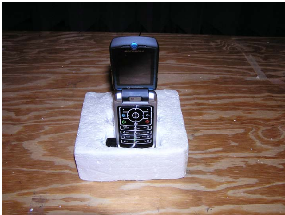
Figure 4. Radiated Emissions X-Axis
