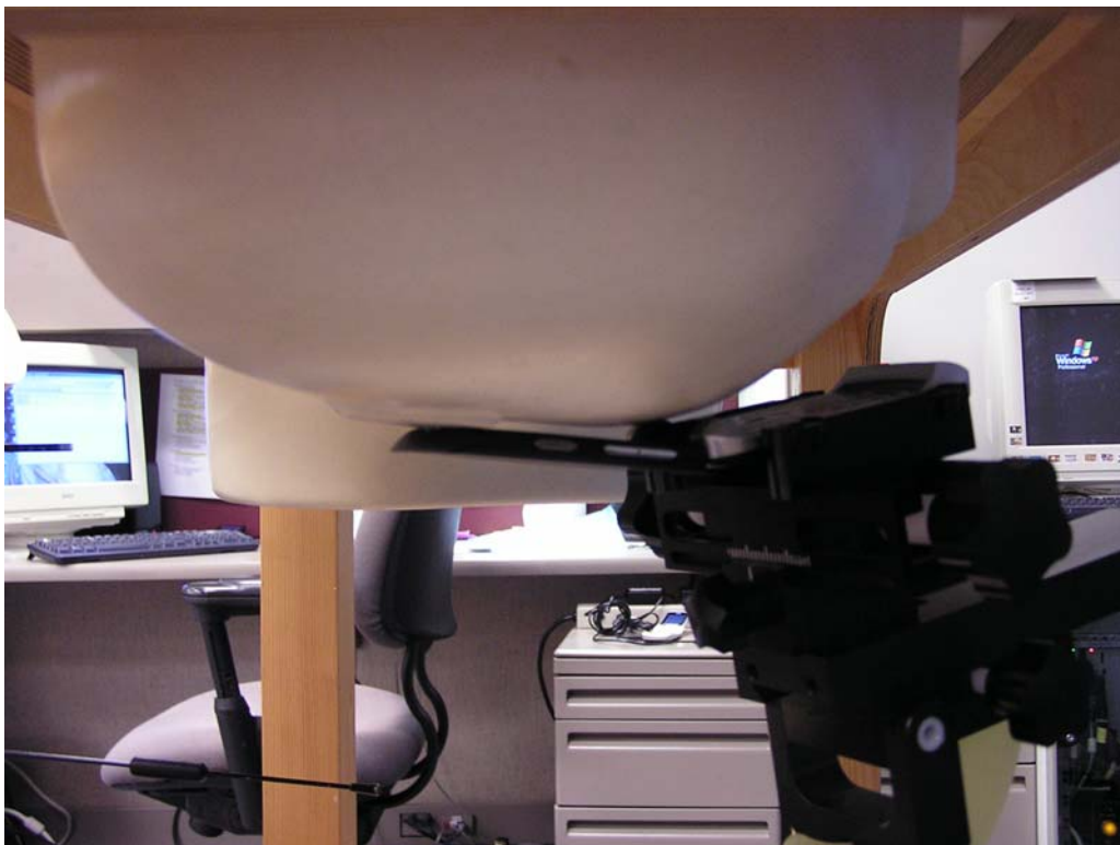
Figure 5 – Transceiver against head, Cheek Touch position
