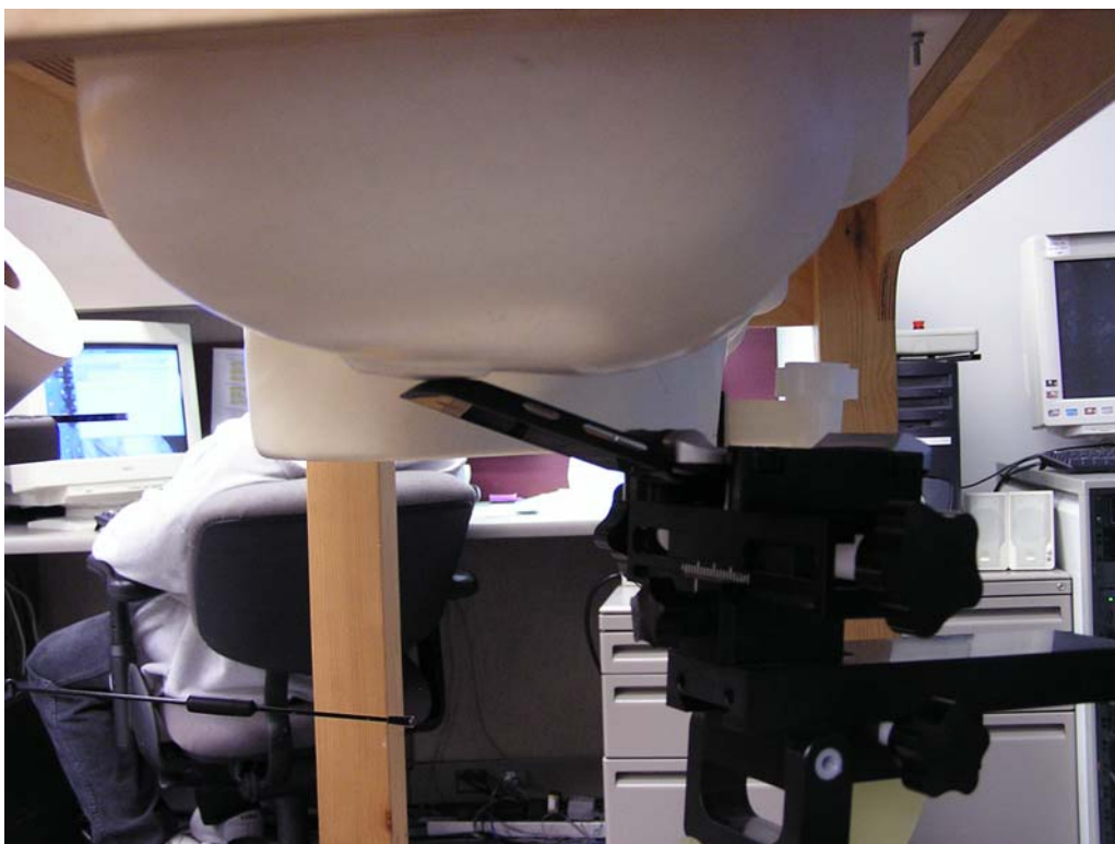
Figure 7 – Transceiver against head, 15° Tilt position
