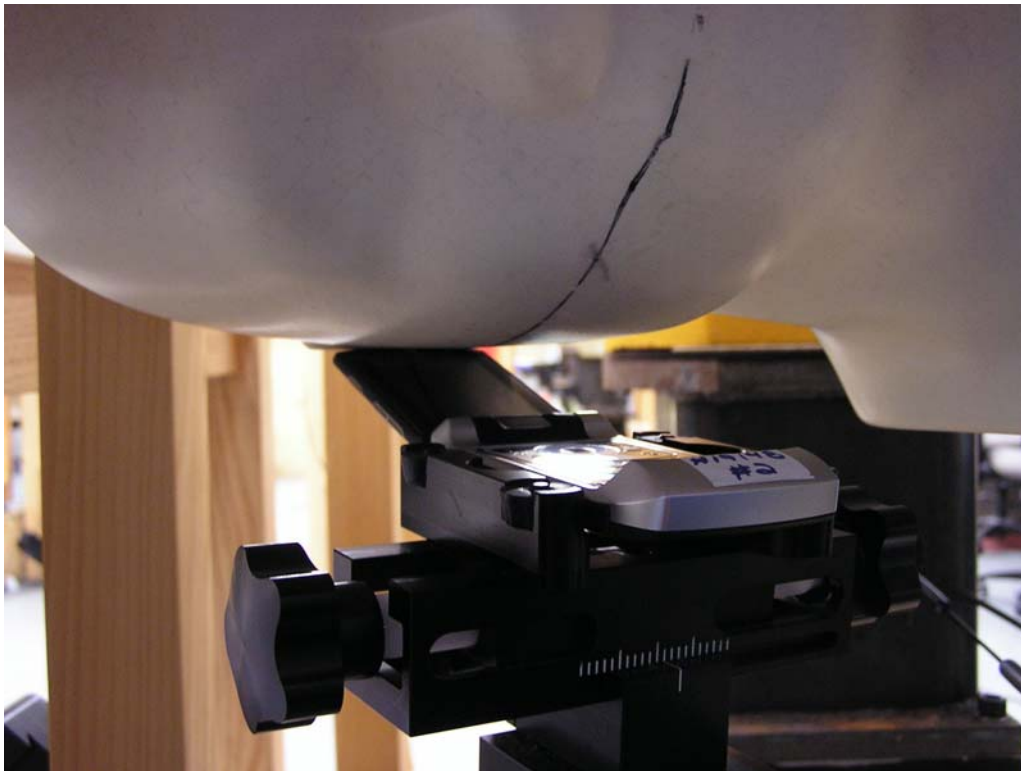
Figure 6 – Transceiver against head, 15° Tilt position
