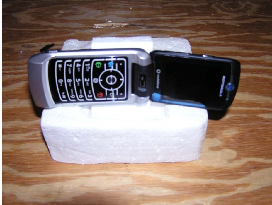
Figure 5. Radiated Emissions Y-Axis
