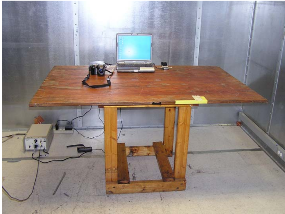
Figure 1. AC Line Conducted Emissions Measurement Setup
