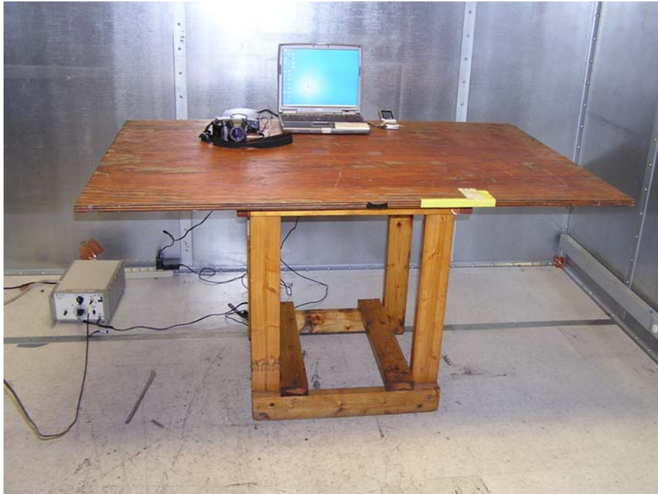
Figure 1. AC Line Conducted Emissions Measurement Setup
