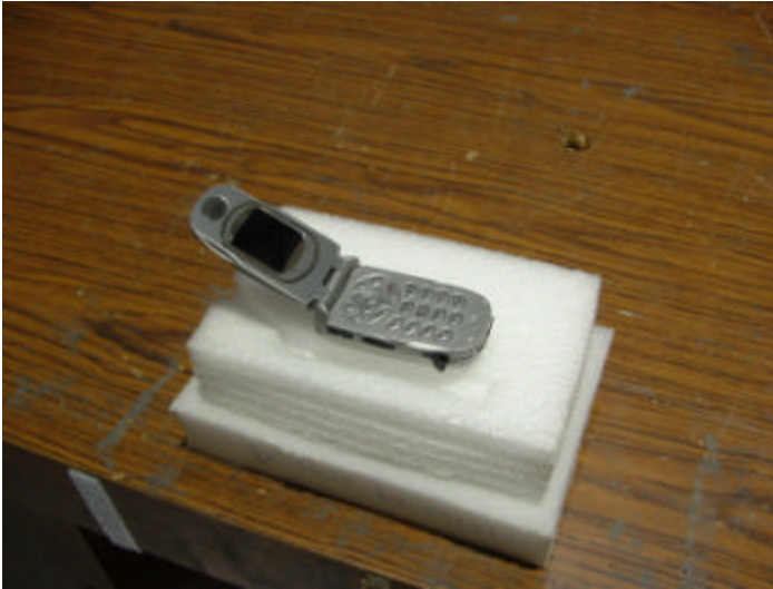
Radiated Emissions Z-Axis
