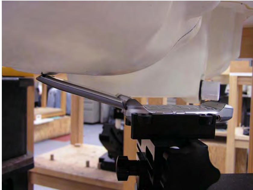
Figure 6. Phone Against the Head Phantom (15°Tilt)
