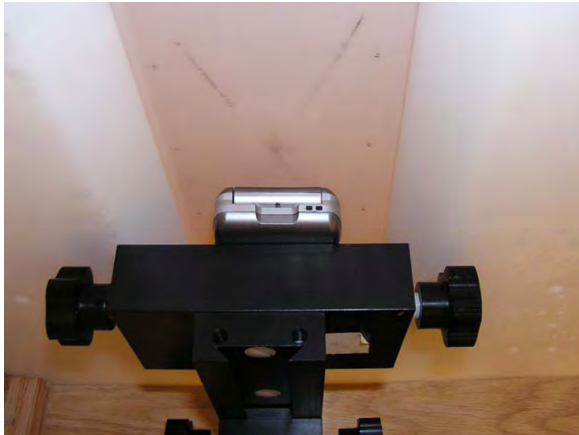
Figure 4. Phone Against the Flat Phantom
