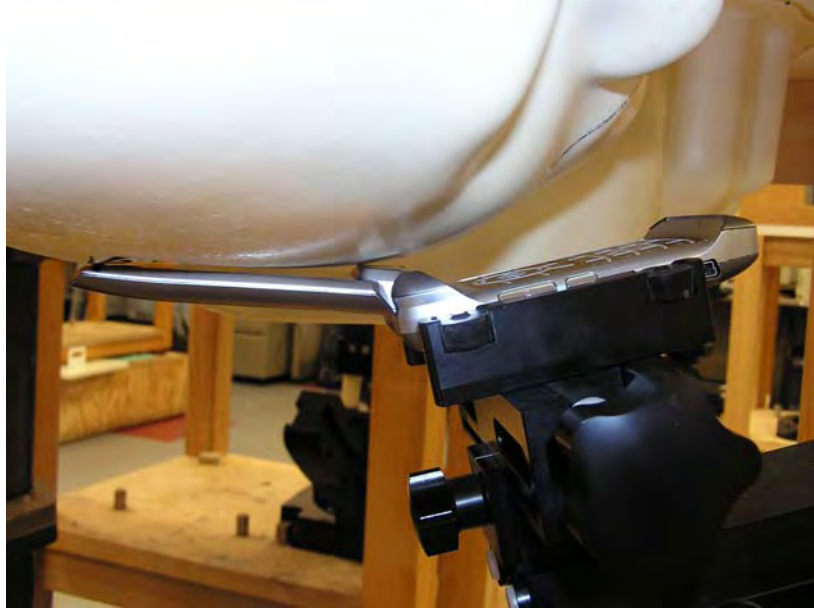
Figure 5. Phone Against the Head Phantom (Cheek Touch)
