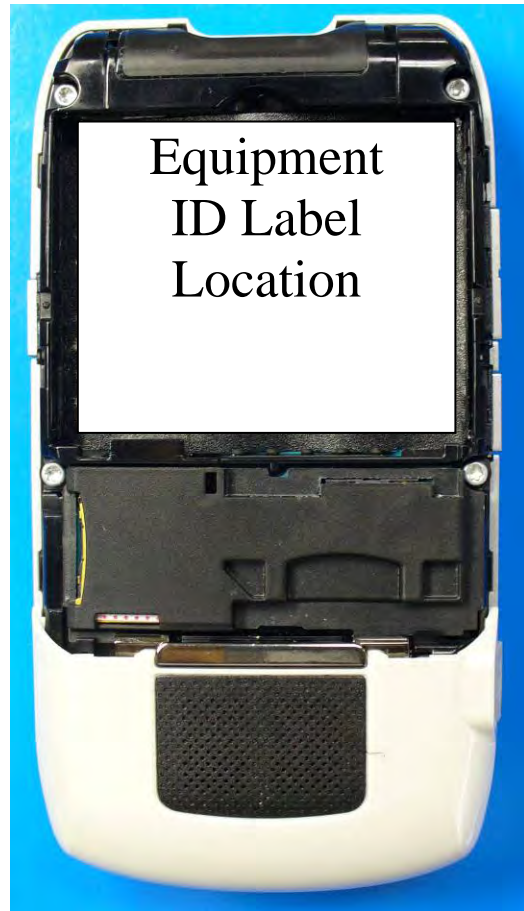
Rear View with Battery removed to show the Equipment ID Label
