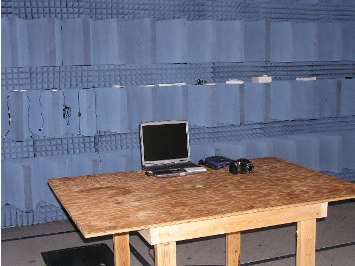
Radiated Emissions Measurement Setup
