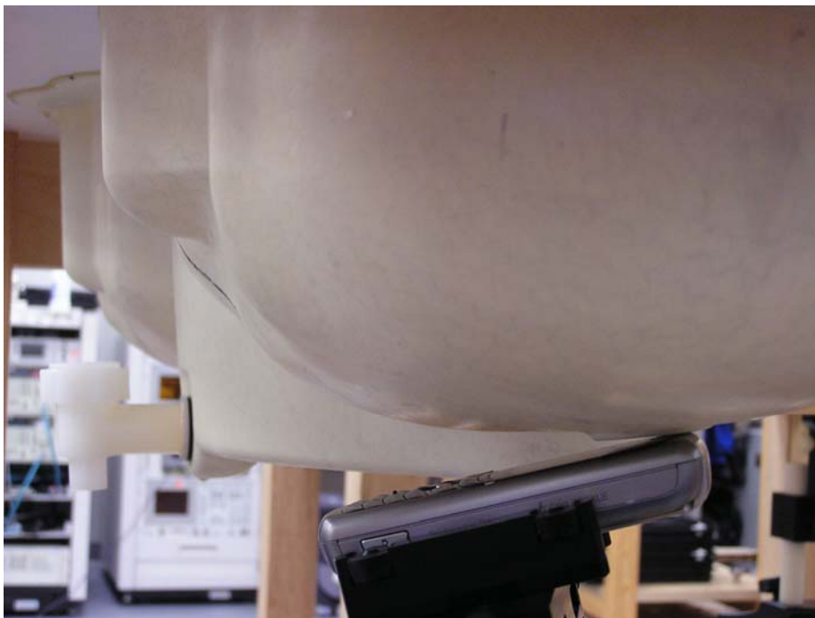
Figure 4. Phone Against the Head Phantom (15°Tilt)
