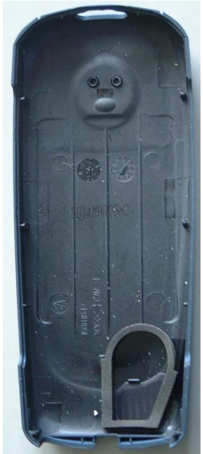
Rear Housing Internal View
