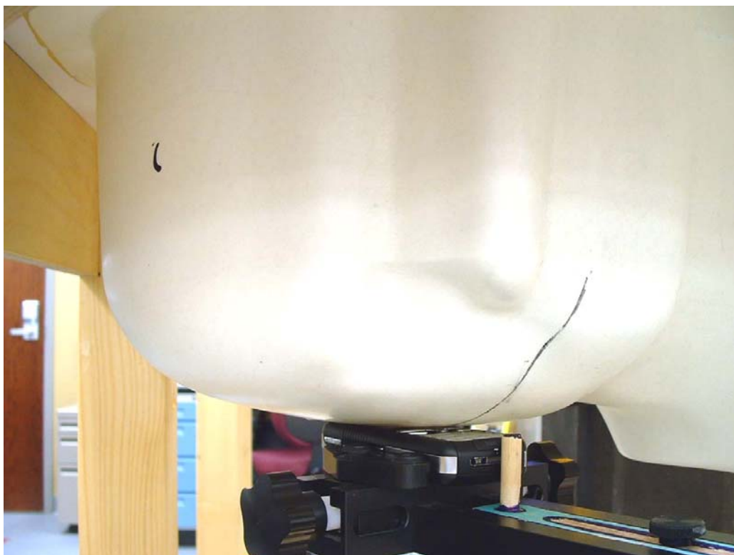
Figure 8. Phone Against the Head Phantom (Front View - Cheek Touch)
