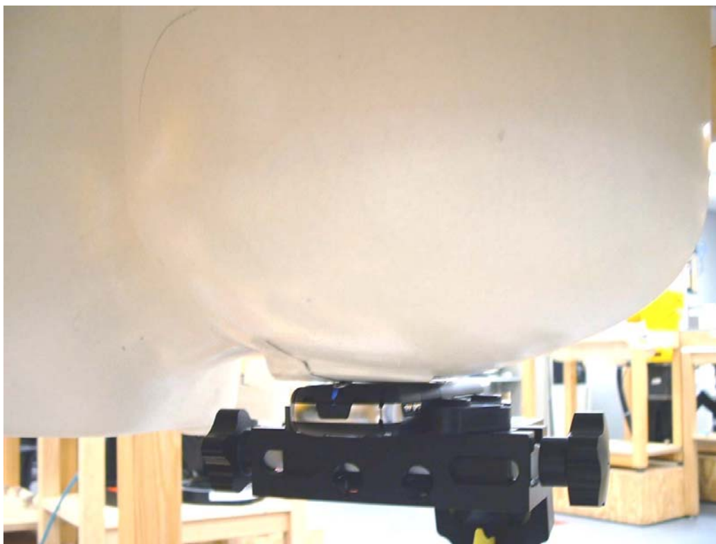
Figure 9. Phone Against the Head Phantom (Back View – Cheek Touch)
