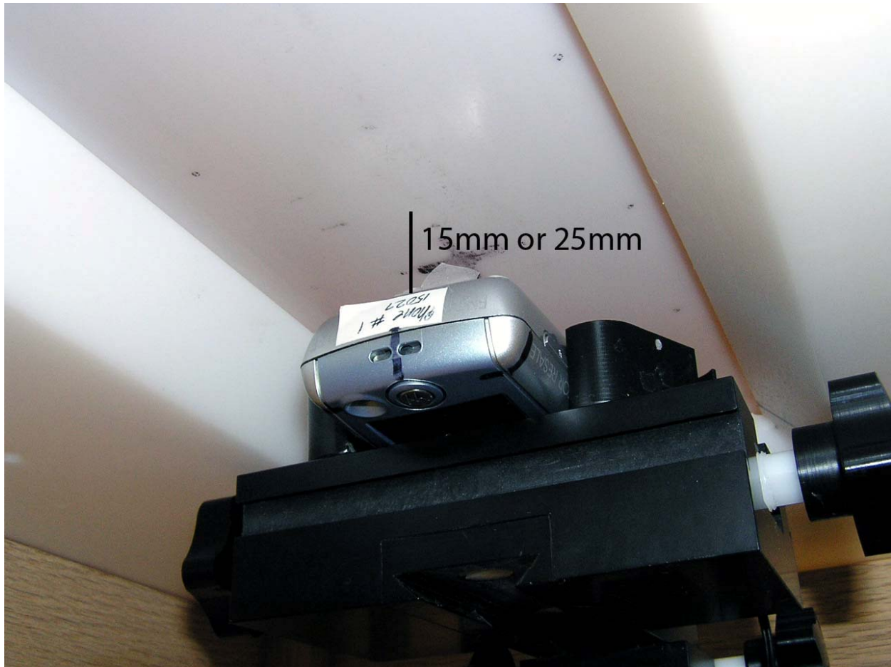
Figure 10. Body Worn testing
