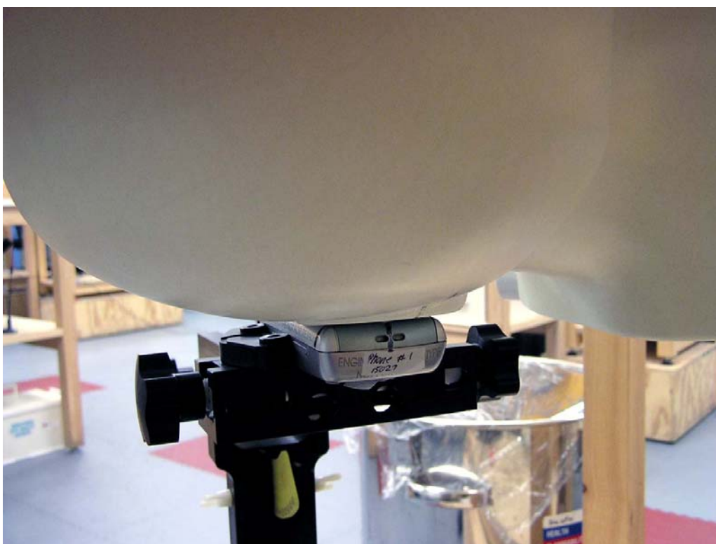
Figure 7. Rear View; Cheek/Touch Position
