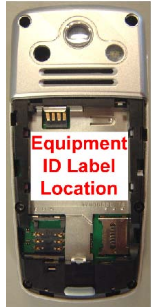
Rear View with Battery Cover Removed Showing ID Label Location
