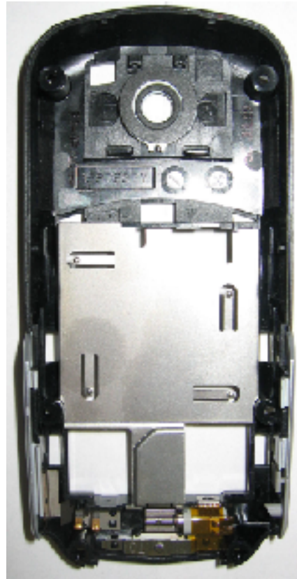
Rear Housing Internal View
