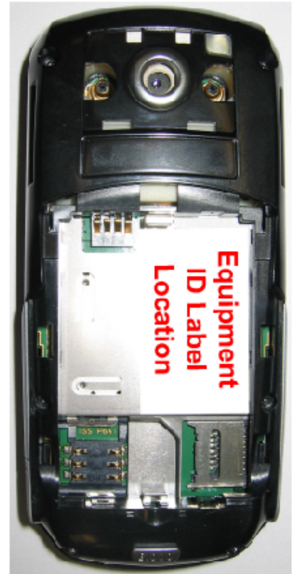
Rear View with Battery Cover Removed Showing ID Label
