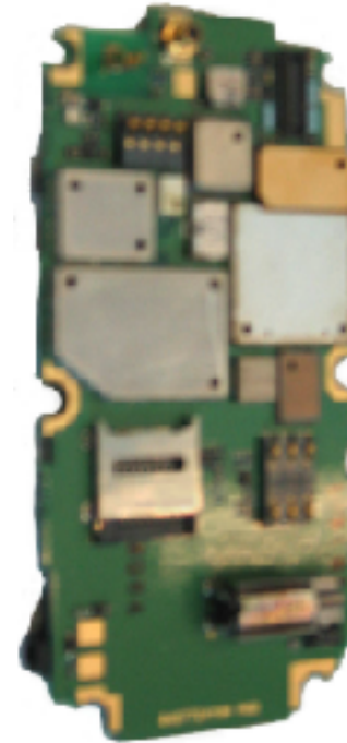
Main Board Rear View (shields on)
