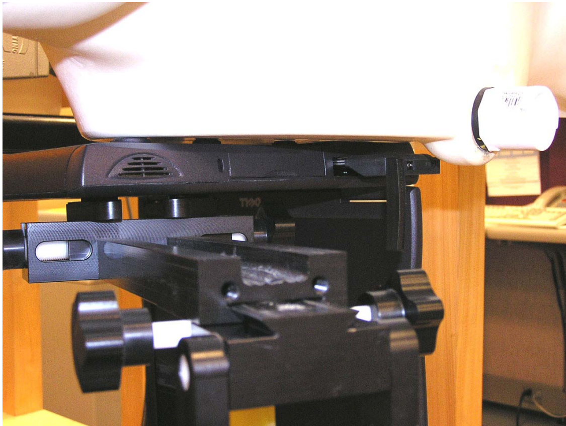
DUT with Antenna Vertical in Dell Latitude C640
