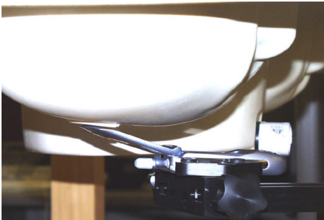
Figure 12. Phone Against the Head Phantom (Back View – 15° Tilt)
