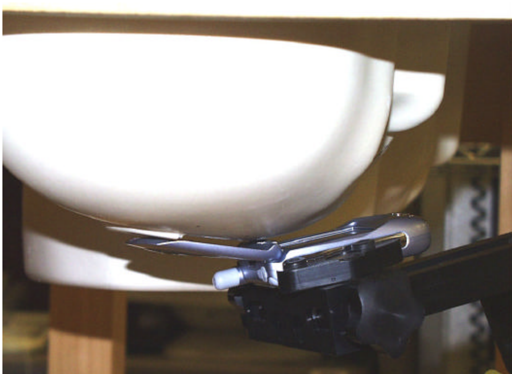
Figure 10. Phone Against the Head Phantom (Back View – Cheek Touch)
