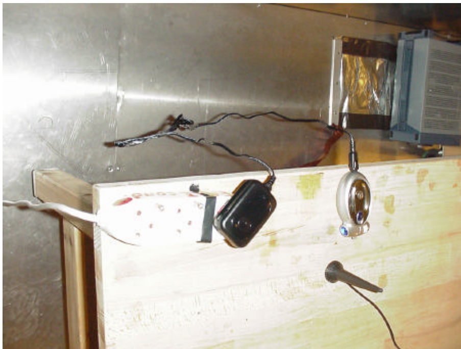
Picture 4 : Setup for conducted emissions tests
