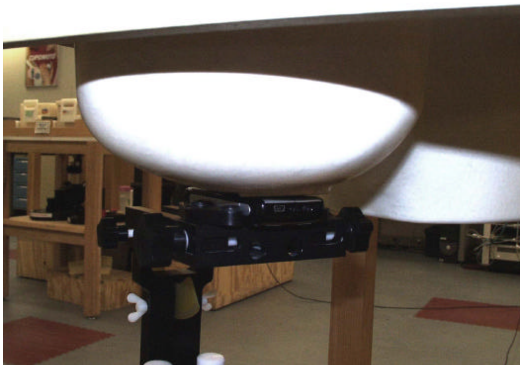
Figure 9. Phone Against the Head Phantom (Back View – Cheek Touch)
